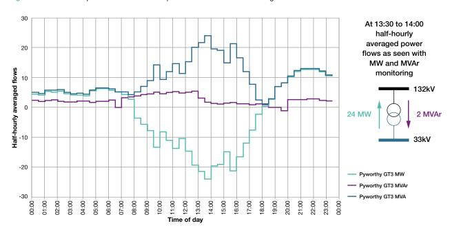
Figure 4: Power flow represented with full four quadrant MW and MVAr metering
