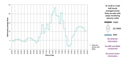
Figure 2: Power flow represented with amps and dummy volts metering
