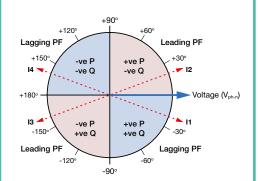
P = active power (kW) Q = reactive power (kVAr)
